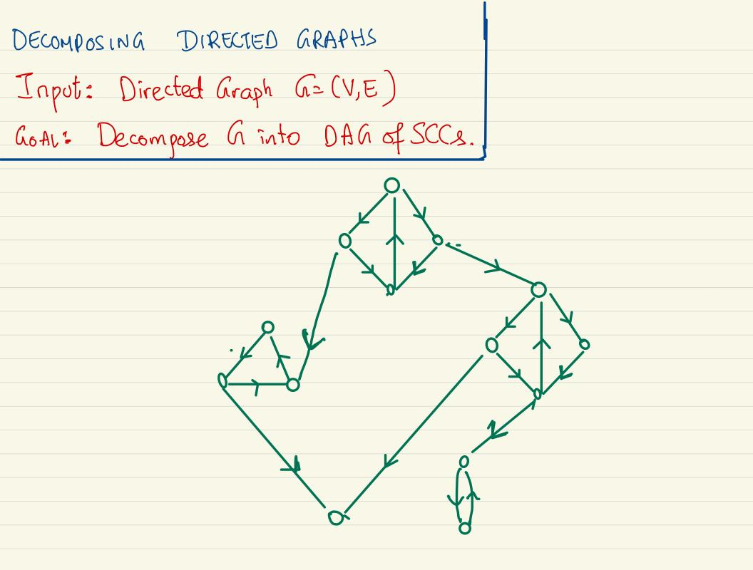
FACT: In a DFS traversal, verter with highest POST value is in a Source Scc. BUT WE WANT: A NODE IN SINK SCC ?? IDEA: 1) RUN DES on GRE G with edges reversed. 2) Output vertex v with HiaHEST POST VALUE V ESOURCESCC in GR = SANSK SCC in GIL
